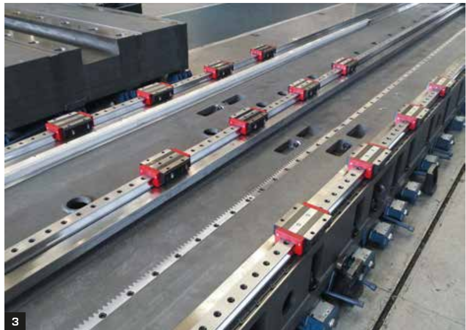
1. Box-in-box design with symmetrical column and vertical stroke on four guides. 2. RAM with four double-sided guides. 3. Maximum precision LM linear guide on the X-Y-Z axes.
