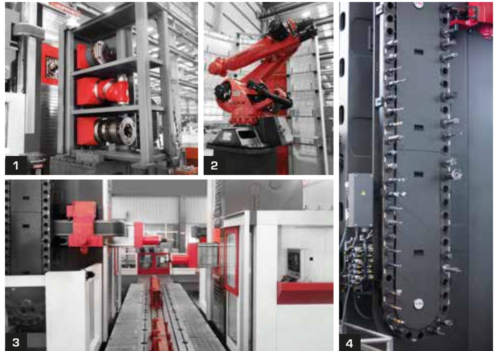
1. AAC Head changer. 2. Robot type ATC tool changer. 3. Duplex configuration. 4. Chain type tool magazine.
