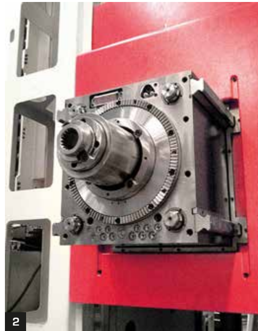
1. Box-in-box design with symmetrical column and vertical stroke on four guides. 2. RAM with four double-sided guides. 3. Maximum precision LM linear guide on the X-Y-Z axes.
