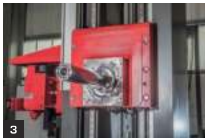
1. Thermo-symmetric structure with central head. 2. Multiple automation options. Detail of the ATC robot. 3. Four-guide vertical head movement: 2 in front and 2 in the rear. 4. Robust structure and high-precision components. 5. Double pinion play-free hydrostatic guide for table rotation.
